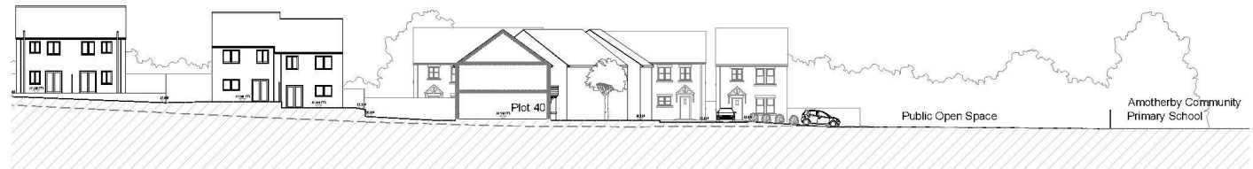
Section to show the development to the North in relation to the new proposed public open space and the existing primary school boundary
