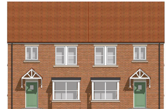
Stonesdale - Arden red brick external wall with red concrete interlocking roofing tiles.
